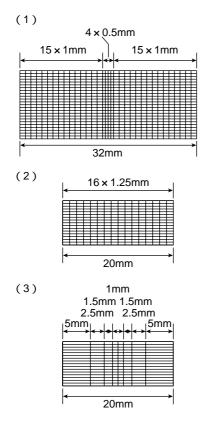
Fig. 1 Multislice CT detectors Matrix type (1, 2) and adaptive array type (3)
