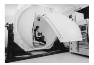
Fig. 4 OVAR system (you can see the inside of the chamber with the door left open.)
