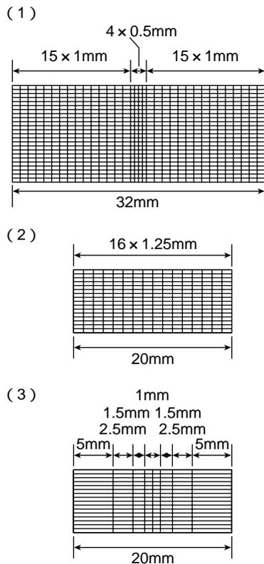
Fig. 1 Multislice CT detectors
